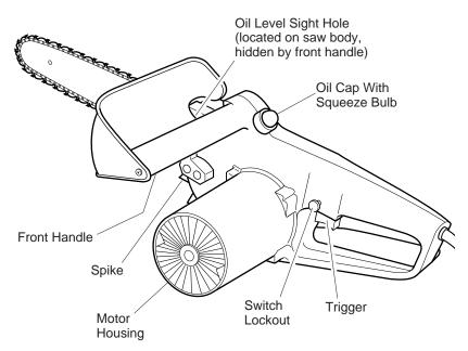
Figure 2 - Electric Chain Saw
